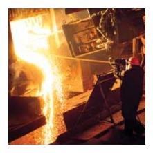
The Electric Arc Furnace (EAF) process has evolved into a highly efficient way to melt scrap metals for steel making. Advances in the technology for injecting various ingredients, including fluxing agents, oxygen, gas and carbon, have led to better energy control and improved process control.
